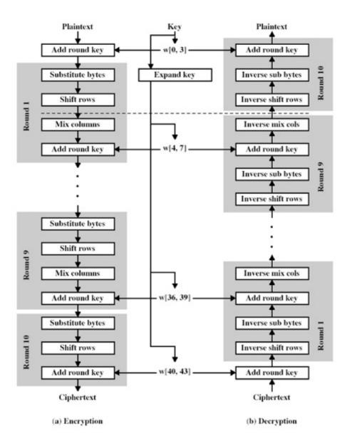
Figure (1): AES Encryption and Decryption
