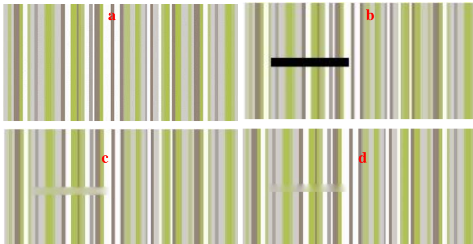
Figure5: Case4 color stripes image, (a) original image, (b) square mask image, (c) image inpainted by isotropic model and (d) image inpainted by modified isotropic model \alpha=1 and \beta=0 .
