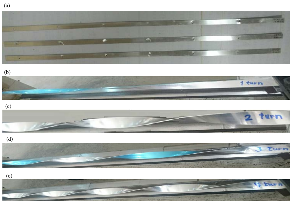
Fig. 2: Different type of tapes with 1-4 twists: a) Hole diameter (4, 7.5 and 10.5 mm); b) 1 twist; c) 2 twist; d) 3 twist and e) 4 twist
