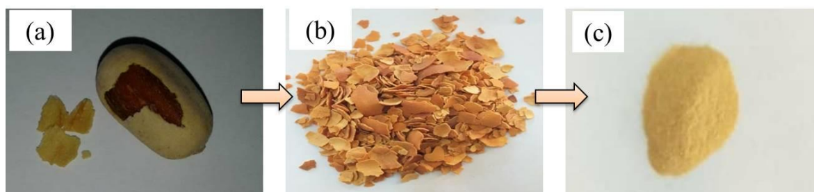
Figure 2. Photographic images. (a) Balanites aegyptiaca "heglig" date; (b) Balanites aegyptiaca seed husks; (c) acid-treated Balanites aegyptiaca seed husks powder (BASHP).
