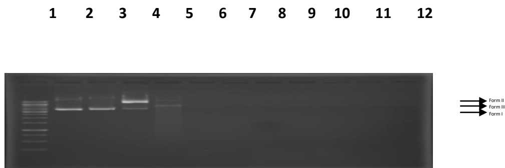
Fig. 12: Cleavage of supercoiled pBR322 (0.5 \mu\text{g}/\mu\text{l} ) at different concentrations of Pd(II) complex in Tris-HCl buffer pH (7.2) for 2 h at 37 ^{\circ}\text{C} . Lane 1: DNA ladder; lane 2: DNA + \text{H}_2\text{O}_2 ; lane 3: DNA + Pd(II) complex (1mM) + DMSO; Lanes: (4-12), DNA with increasing the concentrations of Pd(II) complex (0.1-1mM) + \text{H}_2\text{O}_2 + Buffer.
