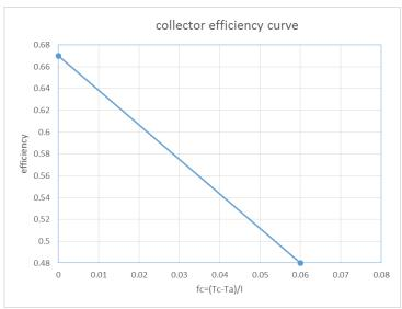
Fig. (5.9). Experimental collector efficiency curve
