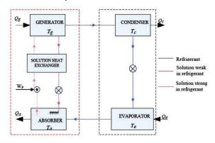
Figure (1.3): Single vapor H<sub>2</sub>O-LiBr absorption cycle
