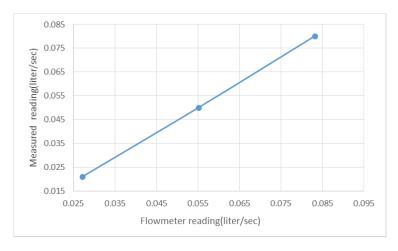
Figure (3.20). Calibration of flowmeter
