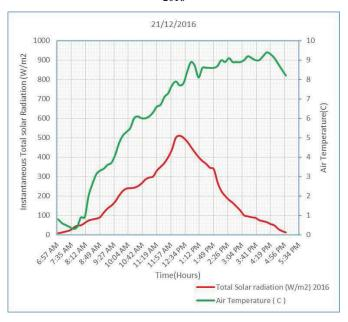
Fig. (5.4) Measured total solar radiation and air temperature at 21stDecember-2016
