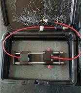
Figure (3.18). A-Transport PT878 flowmeter indicator B-Silicone grease C-Transducer
