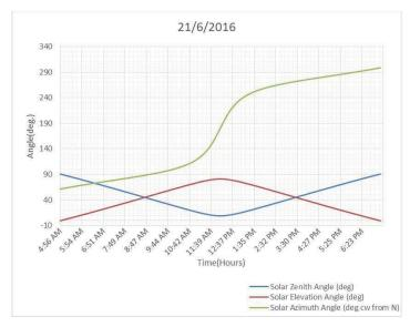
Fig. (5.30) Azimuth angle, zenith angle and elevation angle calculation for June 21 year 2016
