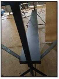
Figure (3.10). Flat plate receiver
