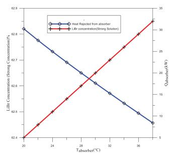
Fig. (541). Heat rejected from absorber unit and LiBr concentration (strong solution) with absorber temperatures
