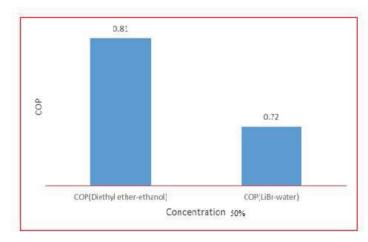
$Fig.\ (5.48)\ Comparison\ between\ COP\ with\ concentration\ (Diethyl\ ether-ethanol)$  and (Lithium bromide-water)
