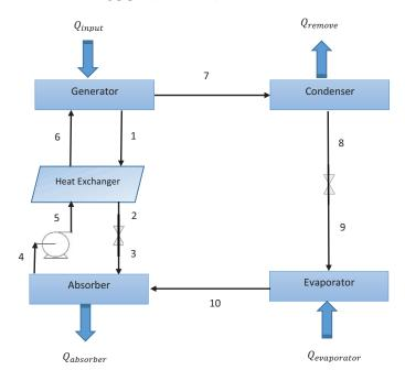
Fig. (4.2) Schematic of an absorption refrigeration process
