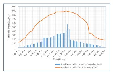
Fig. (5.5) Comparison between measured instantaneous total solar radiation at 21-June and 21-December 2016
