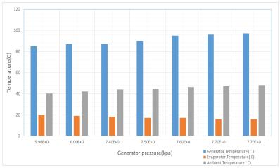
Fig. (5.16). Measured variation of generator, evaporator and ambient temperature with generator pressure at June month, 2016
