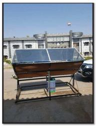
Figure (3.8). Compound Parabolic Collector (CPC)
