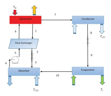
Fig. (4.5) Schematic of an absorption refrigeration process
