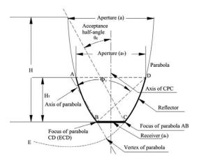
Figure (4.1): Schematic diagram of compound parabolic collector [95]
