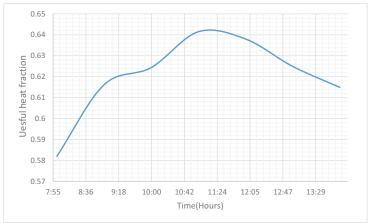
Fig. (5.35). Useful heat fraction from total solar radiation during June month year 2016
