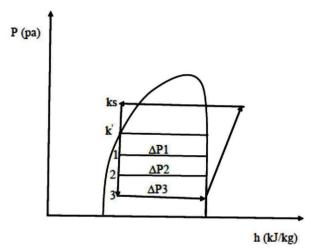
Figure (3.14). P-h diagram of elementary length a long Isenthalpic Line.
