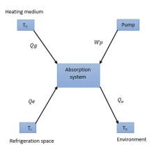
Fig. (4.3) External energy transfers for an absorption refrigeration system
