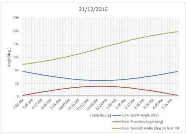
Fig. (5.28) Azimuth angle, zenith angle and elevation angle calculation for 21-December year 2016
