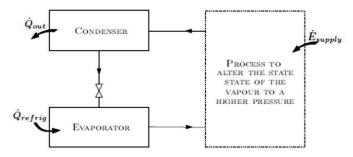
Figure A.1: Generalized refrigeration cycle
