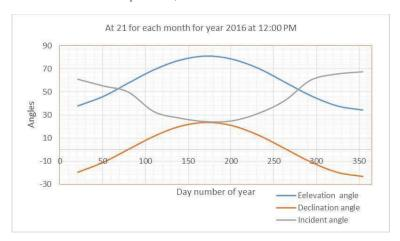
Fig. (5.32) Incident angle, Declination angle and elevation angle calculation at 21st for each month for year 2016
