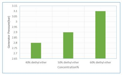
Fig. (5.22). Measured generator pressure with different concentration of diethyl ether  $(July\ 2016)$
