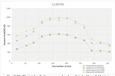
Fig. (5.38). The total radiation measured and predicted with useful heat at different mass flow rate at 21th of each month, year 2016
