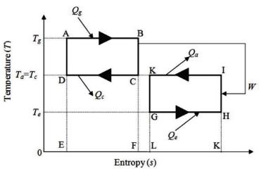
Figure (1.4): Vapor absorption system Muhumuza and Strachan [17].
