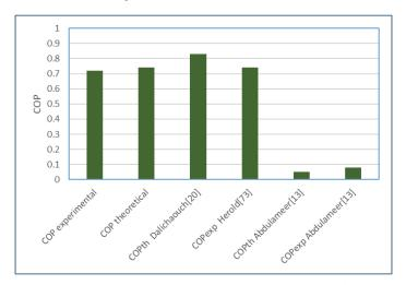
Fig. (5.50). Comparison between experimental, theoretical COP for lithium bromide-water and references [20], [73] and [13]
