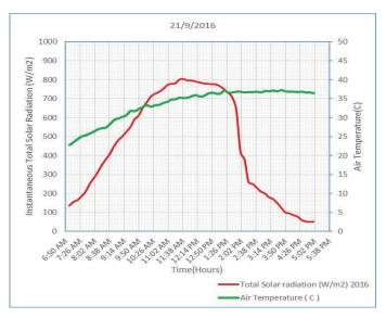
Fig. (5.3) Measured total solar radiation and air temperature at 21st September-2016
