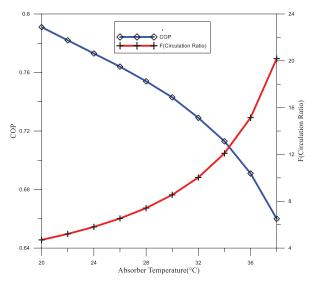
Fig. (5.40). COP of the absorption cooling system and the circulation ratio with absorber temperatures
