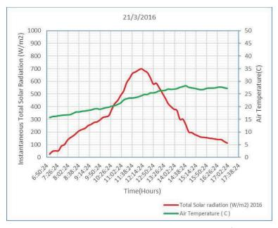
Fig. (5.1) Measured total solar radiation and air temperature at 21st March-2016
