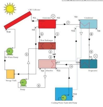
Figure (3.1) Schematic Diagram of Solar Absorption Cooling System
