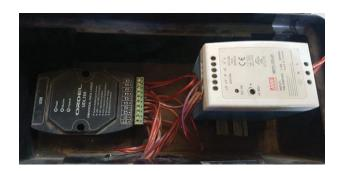
Figure (3.24). Interface and data logger
