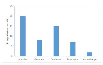
Fig. (5.45) Exergy losses in components
