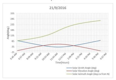
Fig. (5.31) Azimuth angle, zenith angle and elevation angle calculation for 21-September year 2016
