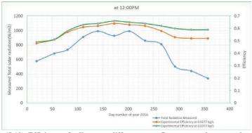
Fig. (5.10). Efficiency of collector at different mass flow rates and measured total solar radiation at 21st for each month at 12:00 pm year 2016
