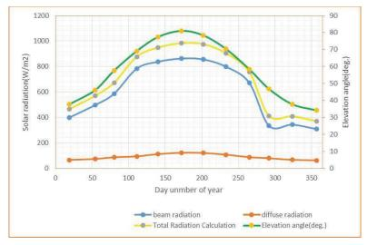
Fig. (5.27) Total solar radiation, beam solar radiation, diffuse solar radiation and elevation angle for the 21<sup>th</sup> day of each month at 12:00pm, year 2016
