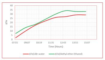
Fig. (5.47) Comparison between evaporator temperature difference with time for (Diethyl ether-ethanol) and (Lithium bromide-water) at same concentration 50% for June 2016
