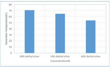
Fig. (5.21). Measured generator temperature with different concentration of diethyl ether (July 2016)
