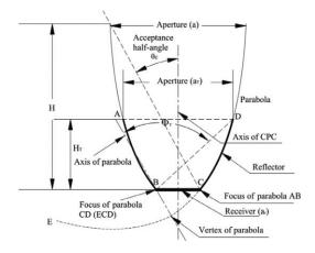
Figure (3.2). Full Compound Parabolic Concentrator [94]
