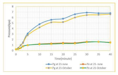
Fig. (5.13). Measured variation of pressure of generator and evaporator with time at  $21^{\rm th}$  of June and October 2016
