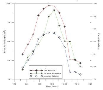
Fig. (5.39). Predicted solar radiation and  $\,$  hot water temperature with Time at  $21^{th}$  of June 2016
