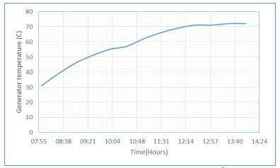
.Fig. (5.19). Experimental generator temperature with time at 21th of July 2016
