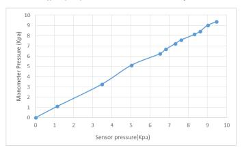
Figure (3.22). Pressure calibration
