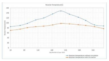
Fig. (5.8). The collector receiver temperature at 21<sup>th</sup> of each month at 13:00 pm, with and without hot water circulation, year 2016
