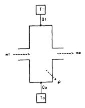
Fig. (4.6) Open system in thermal contact with *n* heat reservoirs [20]
