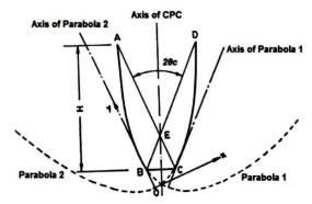
Figure (1.2): Cross section of a symmetrical non-truncated CPC Winston et al [11].
