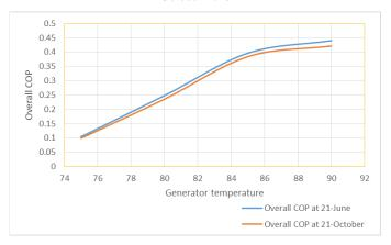
Fig. (5.18). Experimental overall COP with generator temperature at 21<sup>th</sup> of June and October 2016
