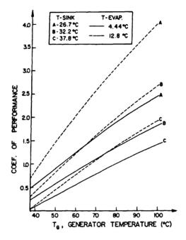
Fig. (4.8) System COP of an ideal absorption cycle [20]
