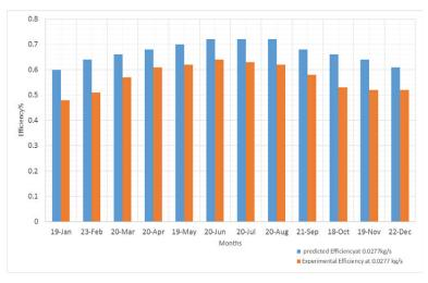
Fig. (5.37). The theoretical and experimental efficiency of collector at mass flow rate 0.0277kg/s.
