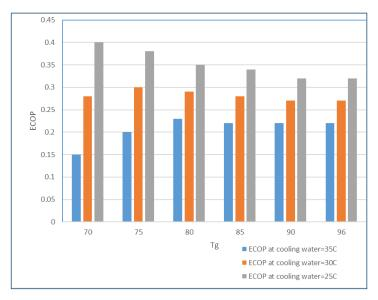
Fig. (5.46) Exergy efficiency of the absorption refrigeration system with the generator temperature for different cooling water temperatures
