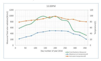
Fig. (5.11). Measured instantaneous total solar radiation, ambient temperature and hot water temperature during year 2016
