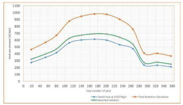
Fig. (5.34) Total solar radiation, absorbed radiation and useful heat at different mass flow rate at 12:00pm for year 2016
