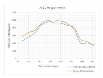
Fig. (5.25). Annual max. Daily radiation the measured total solar radiation and predicted at  $21^{\text{th}}$  of each month
