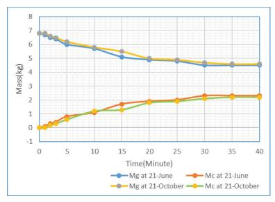
Fig. (5.14). Measured variation of mass in generator and condenser with time at  $21^{\rm th}$  of June and October 2016
