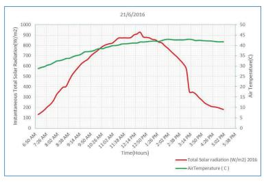
Fig. (5.2) Measured total solar radiation and air temperature at 21st June-2016
