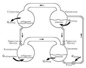
Figure (2.3): Absorption principle, part three absorption and generation of vapor combined for a complete cycle Dawood [32]
