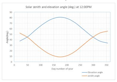
Fig. (5.33) Zenith and elevation angle calculation at 12:00pm for year 2016
