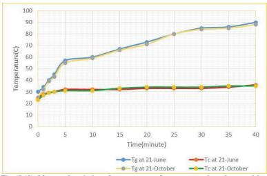
Fig. (5.12). Measured variation of temperature of generator and condenser with time at 21<sup>th</sup> of June and October 2016
