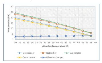
Fig. (5.42). Heat amount with absorber temperatures
