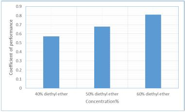
Fig. (5.23). Measured coefficient of performance with different concentration of diethyl ether (July 2016)
