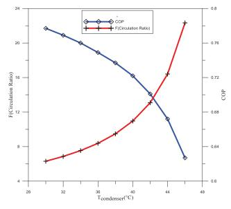
Fig. (5.43). COP of the absorption cooling system and the circulation ratio with condenser temperatures
