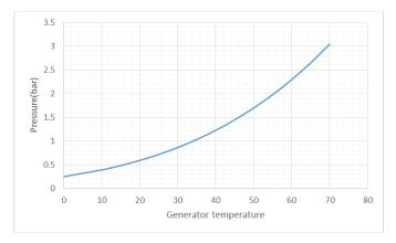
Fig. (5.44). Generator pressure vs generator temperature for Diethyl ether
