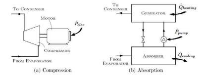
Figure A.2: Comparison of components used for the conditioning of refrigerant vapor through a compression and absorption process
