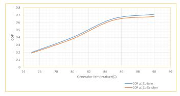
Fig. (5.17). Experimental COP with generator temperature at 21<sup>th</sup> of June and October 2016
