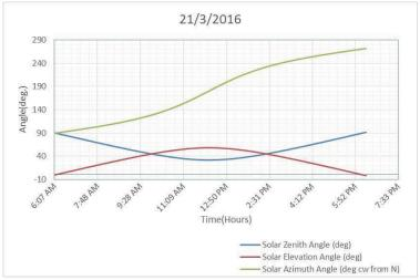
Fig. (5.29) Azimuth angle, zenith angle and elevation angle calculation for 21-March year 2016
