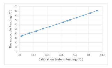
Figure (3.21). Calibration of the Thermocouple
