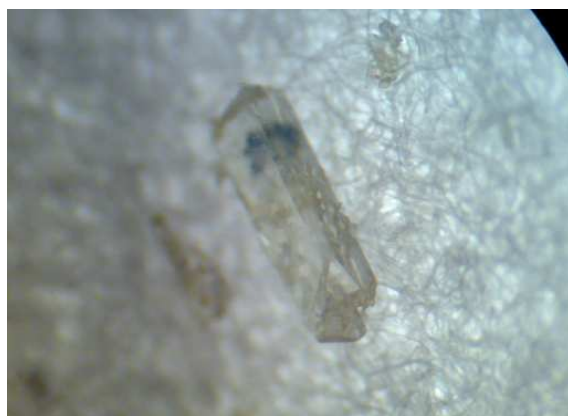
Figure ( 1 ) : Needle crystal of piperine 16 x
