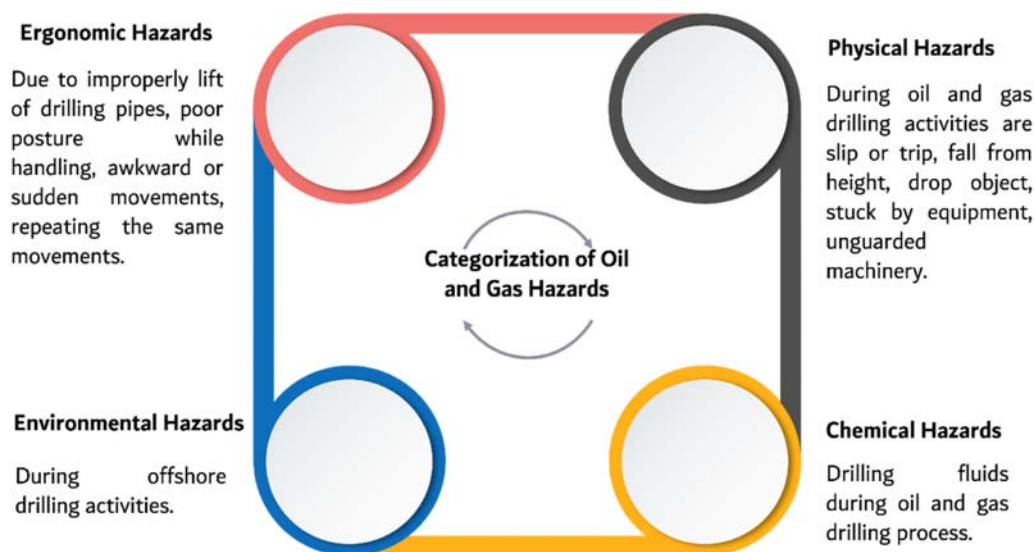
Figure 9.1 Oil and gas hazards categorization.
