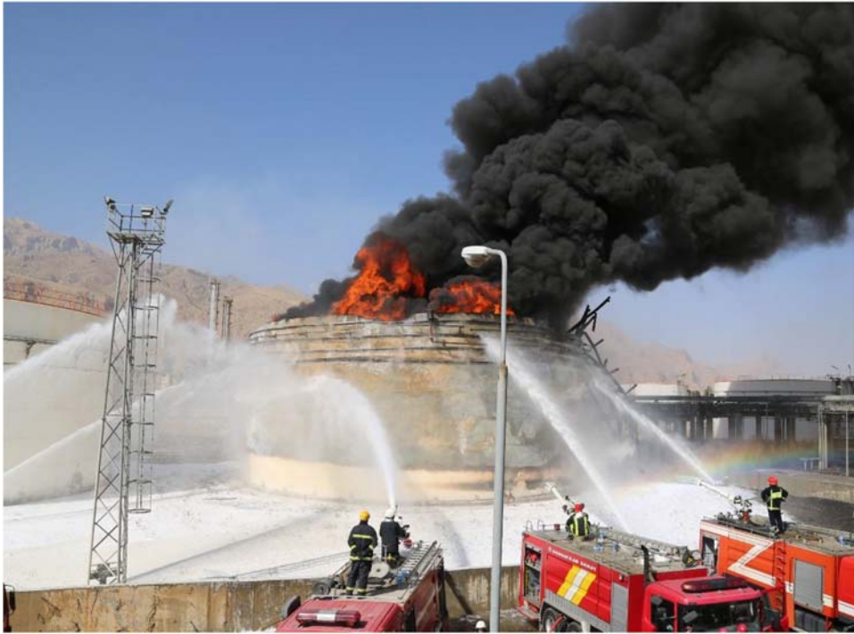
Figure 7.7 Tank wall cooling operation.
