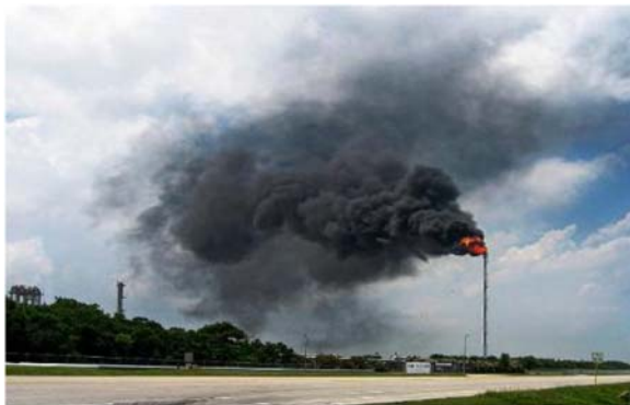
Figure 14.3 Burning gas flare with a huge amount of waste gas, Bayport industrial District, Harris County, Texas [27].
