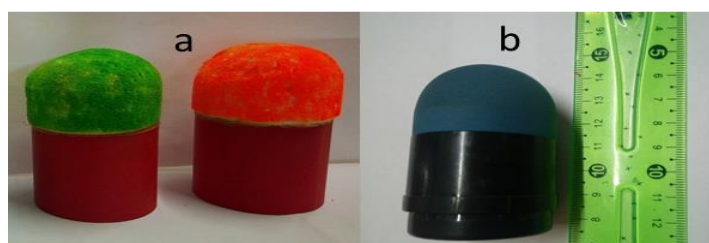
Fig 1. a- Range of specimens elaborated respectively on the non-lethal projectile polyurethane foam b- Specimen referenced XM1006 non-lethal projectile
