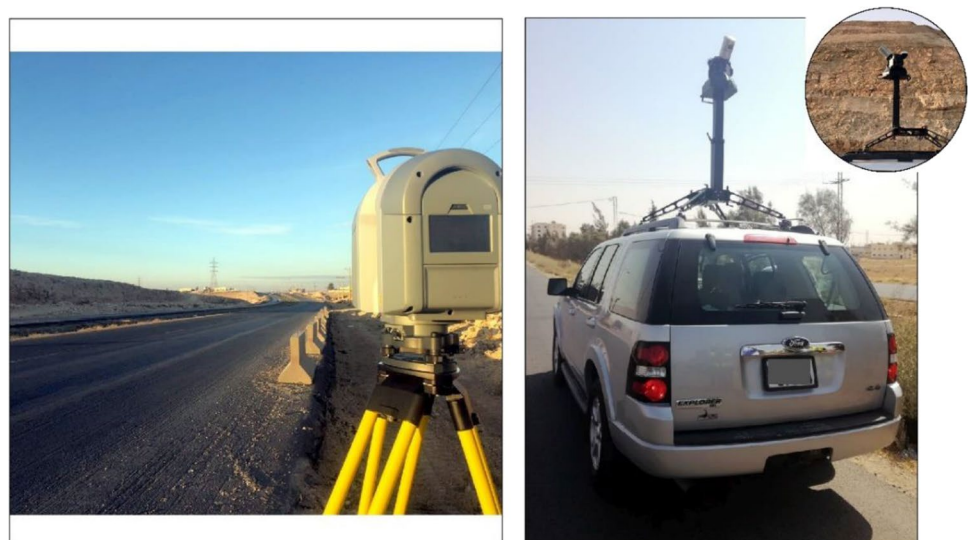
Fig. 4 Data collection systems used in the study (left, static laser scanner; right, mobile laser scanner)
