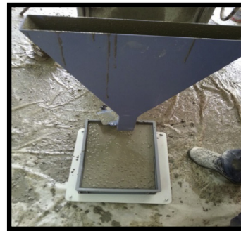
b: V-funnel flow time test
