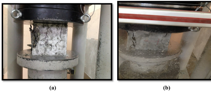
Fig. 10. (a) Cubic failure under compressive force test for with FPW. (b) Cubic failure under compressive force test for with CPW.
