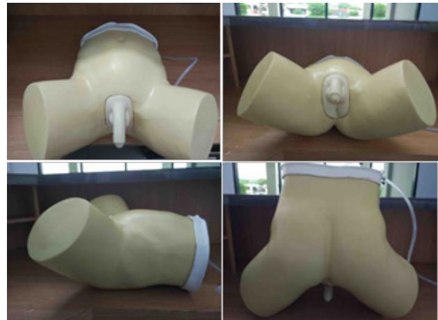
Figure 1. Outer part of male catheterization mannequin
