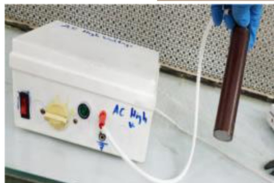
Fig. 2. Large Probe of the Proposed FE-DBD.
