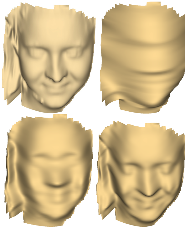
Figure 5.4: Polynomial interpolation degrees 3 to 15. The top row left: original face model with a file size of 4MB; the top right, with polynomial interpolation of degree 3 reducing the file size to 8KB. Bottom row left: polynomial degree 10 reducing the file size to 16KB; bottom right, degree 15 reducing to 25KB.
