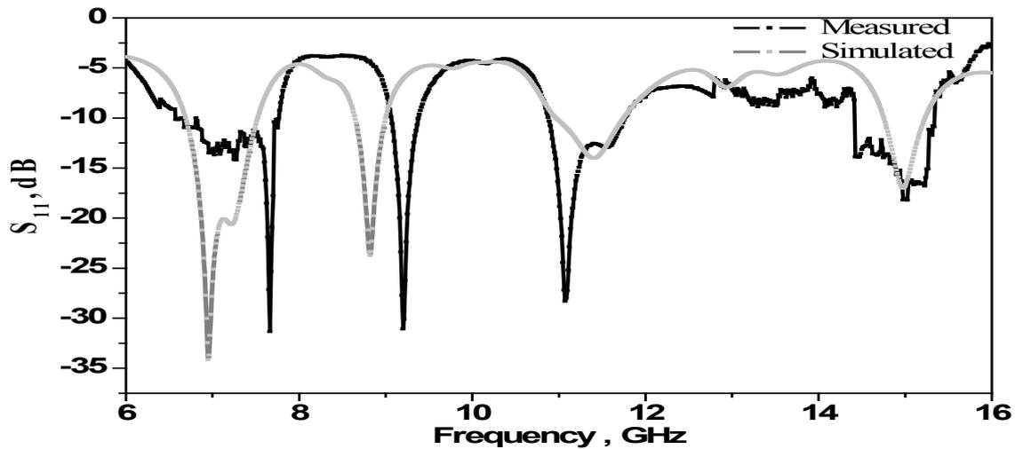
Figure 15 Comparison between the simulated and measured  $S_{11}$  of the proposed antenna array  $1 \times 4$ .
