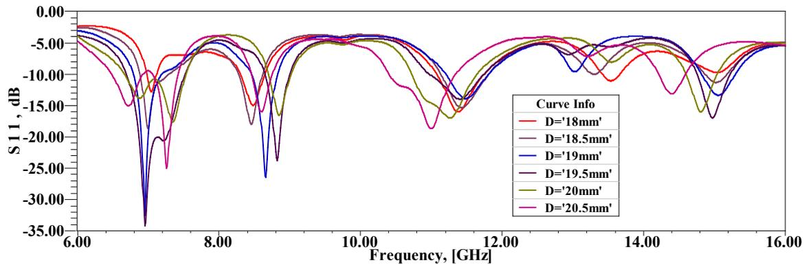
**Figure 13** Effect of mutual coupling in H-plane on antenna array parameters.
