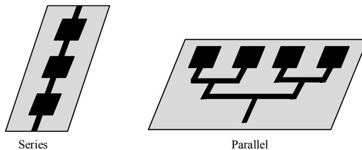
**Figure 4** Feeding of a one-dimensional array.
