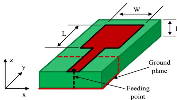
**Figure 1** Geometry of the patch antenna.
