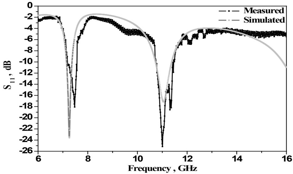
**Figure 9** Comparison between the simulated and measured  $S_{11}$  of the proposed antenna element.
