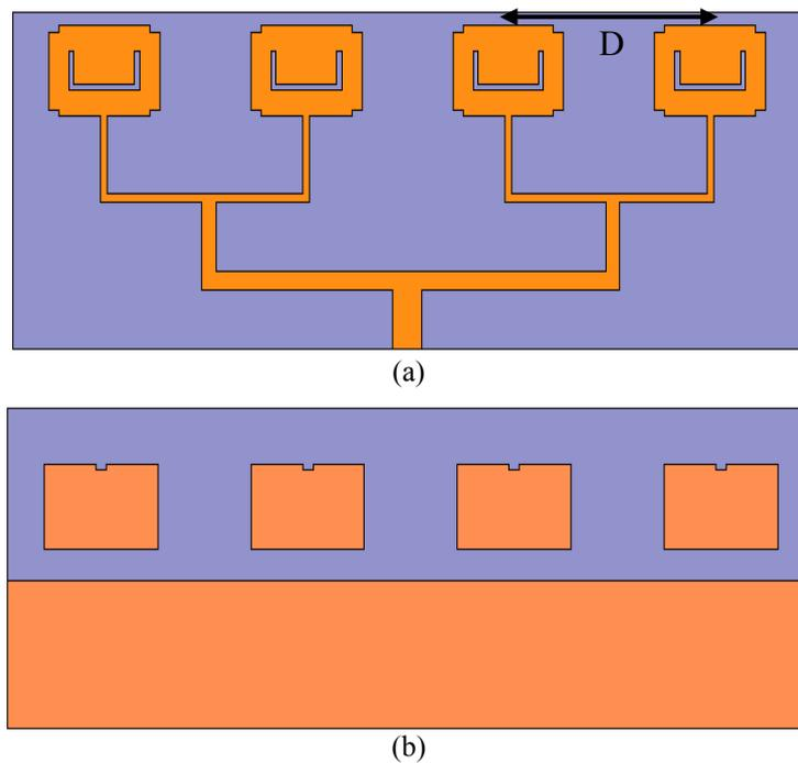
Figure 12 Geometry of the antenna linear array, (a) Top view, (b) Bottom view.
