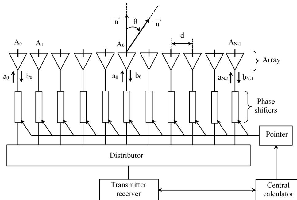
**Figure 2** General structure of a linear array.
