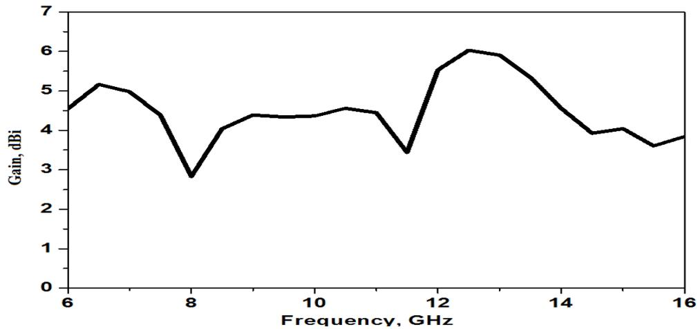
Figure 11 Gain of the antenna at different frequencies.
