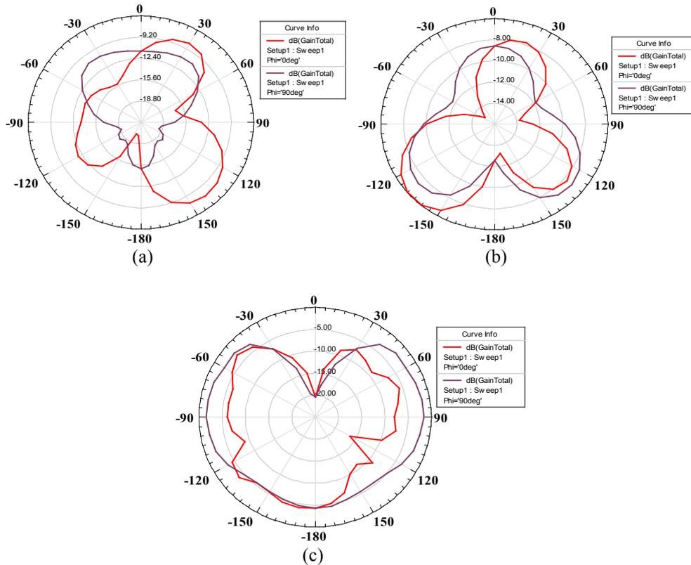
**Figure 10** E-Plane and H-Plane Radiation patterns of the proposed antenna at different frequencies: (a) 7.26 GHz, (b) 11.03 GHz, and (c) 15.96 GHz.
