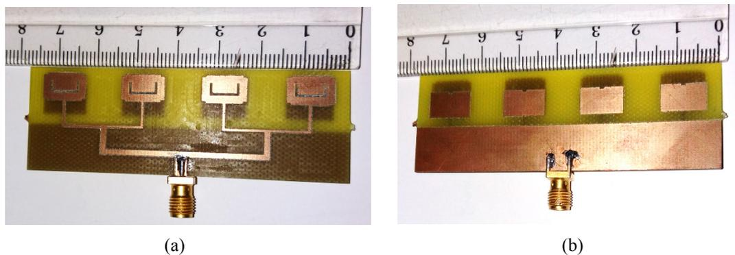
**Figure 14** The fabricated antenna array  $1 \times 4$  (a) Top view, and (b) Bottom view.
