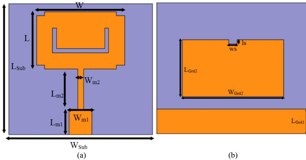
**Figure 6** Geometry of the proposed antenna, (a) Top view, (b) Bottom view.
