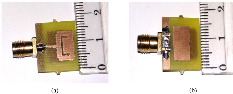
**Figure 8** The fabricated antenna element (a) Top view, and (b) Bottom view.
