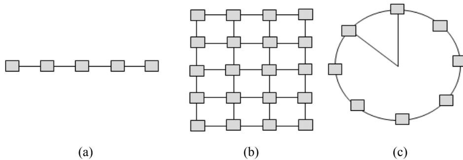
**Figure 3** Different geometric configurations of the arrays, linear (a), 2-dimensional (b), and circular (c).
