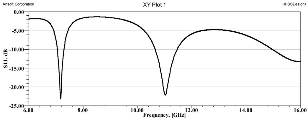
**Figure 7** Return loss of the proposed antenna.
