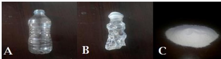
Figure 4. PET used (A) Disposable Bottle, (B) melted waste PET (C) Granules of waste PET.
