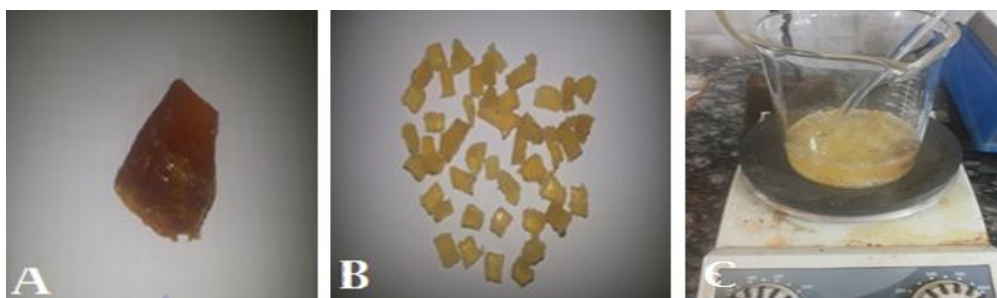
Figure 5. (A) Natural Rubber NR, (B) Small pieces of natural rubber (C) Natural rubber after dissolution
