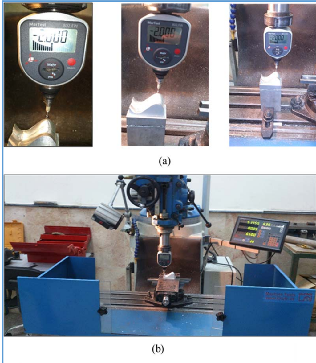
Figure 3.29: Workpiece dimensions measurement, (a) Digital 3D-Touch Probe, (b) Knuth MF1 vertical milling machine.
