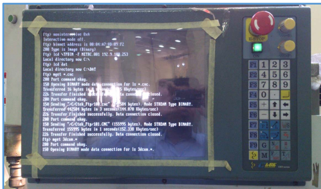
Figure (4.20): C-tek KM-80D Vertical Machining display shows information about wireless file transfer.
