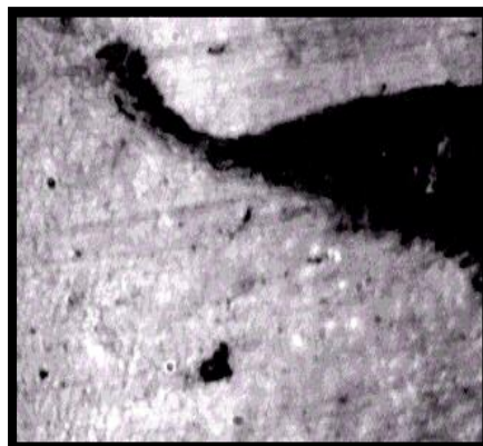
Figure (18) joining between the two metals (X125)
