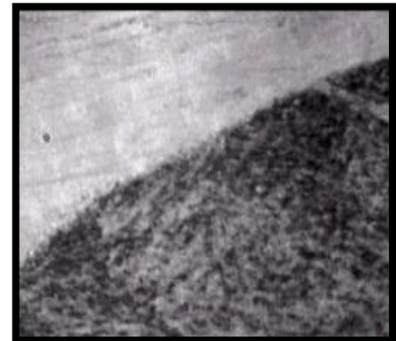
Figure (13) weld joint of St. to St. St. (X 125)
