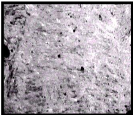
Figure (12) the HAZ with the MW (X 125)
