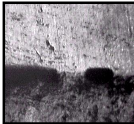
Figure (7) the leak of joint between St. & St. St. (X125)
