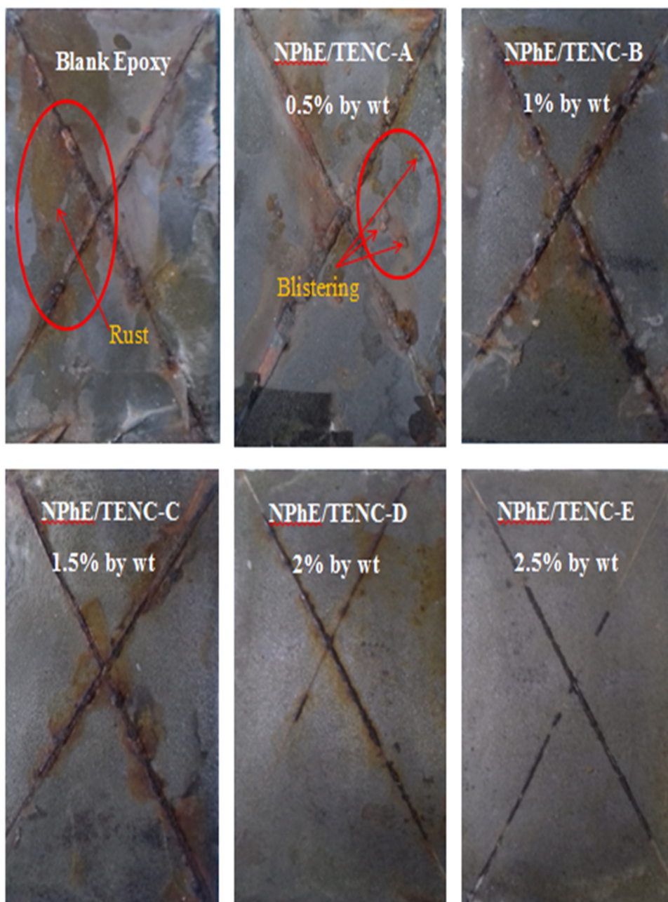
Fig. 5. Salt spray test for the investigated unmodified and various modified NPhE/TNC epoxy coated films after direct exposure to 5% NaCl solution for 500 h at 35 °C.
