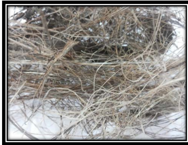
Fig.(1) Palm fiber taken from the rules of palm leaves after cleaning operations performed annually
