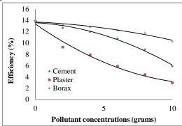
Fig.5: The impact of pollutant accumulation on the PV cell efficiency
