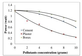
Fig.4: The impact of pollutant accumulation on the PV cell power
