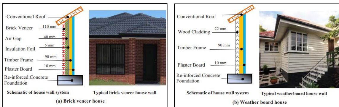
Figure(4): Brick veneer and weather board walls in Australia (Traditional method). Source: [55]
