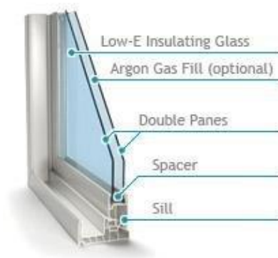
Figure(2): Double glazed windows Source: [37]
