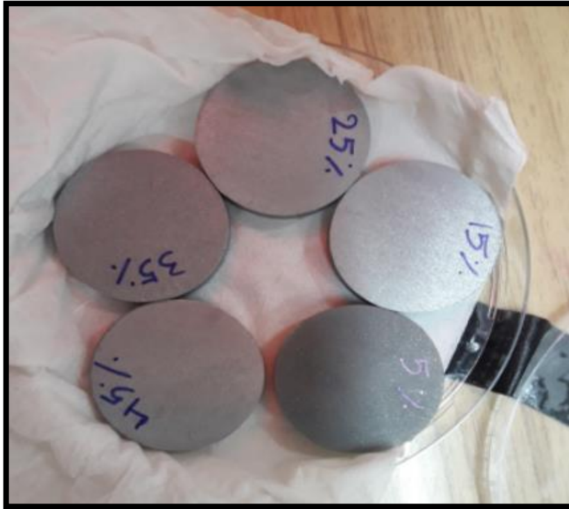
Figure Photograph of Thermal conductivity Test Specimens for Epoxy/ Aluminum composites.
