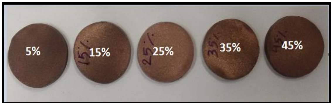
Photograph of Electrical Test Specimens for Epoxy/ Copper composites.
