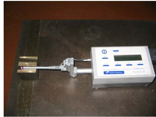
(b) Stylus-based profilometer (Surtronic 3+)
