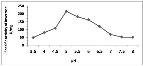
**Figure 5-** Effect of pH on invertase production from *S. cerevisiae*, using wheat bran, incubation for 4 days at 30 °C.
