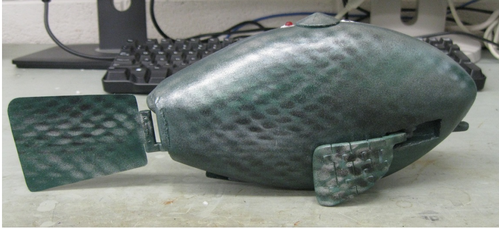
Figure 2.8: The museum robotic fish prototype developed in the Smart Microsystems Lab at Michigan State University.
