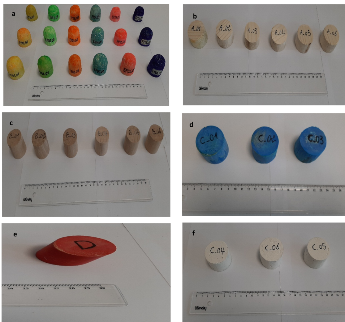
Figure 2. General appearance of dynamic testable samples: (a) Six optimized formulas of nonlethal projectiles in polyurethane foam; (b) Samples of natural beechwood; c. Samples made of artificial plywood; d. Samples of nonlethal projectile holders made of acid polylactic (PLA); e. Samples of nonlethal projectile holders made of acrylonitrile butadiene styrene (ABS); f. Samples of nonlethal projectile holders made of high-density polyethylene (HDPE).
