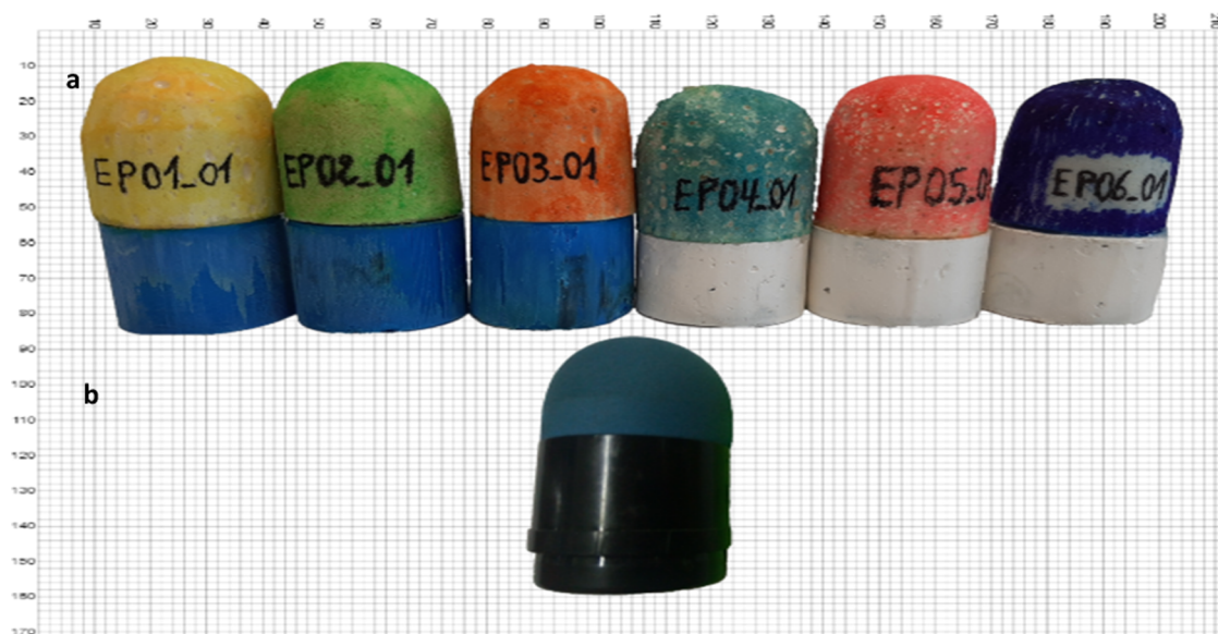
Figure 3. a. Range of specimens elaborated on nonlethal projectile polyurethane foam. b. Specimen referenced XM1006 nonlethal projectile.
