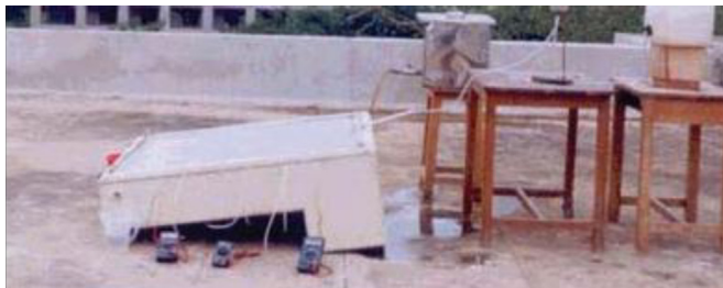
Fig. 17. The experimental still.
