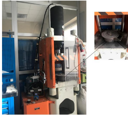
Figure 5. Overall view of hydrostatic pressing machine
