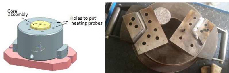
Figure 6. ECAP Die geometry and 120° intersected channels.
