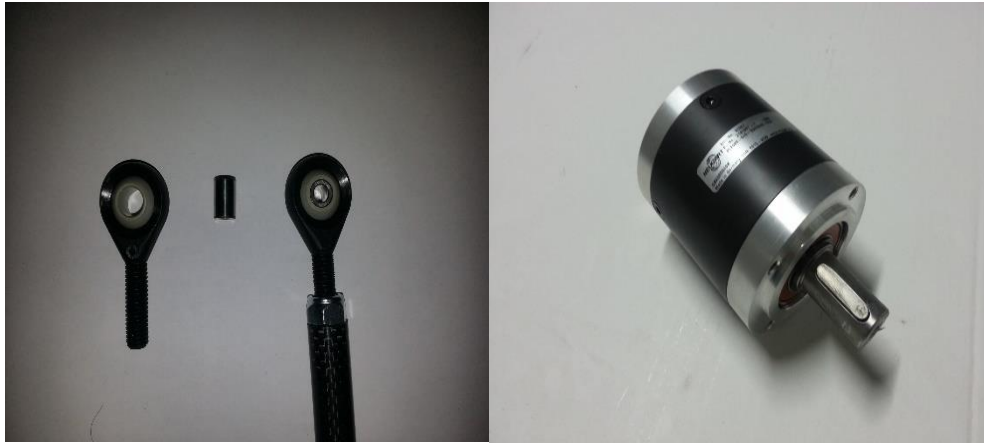
Figure 5. Other mechanical components (left: joint, right: planet-reducer)
