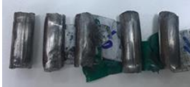
Figure 7. Typical appearance of ECAPed sample billets of Al7075.
