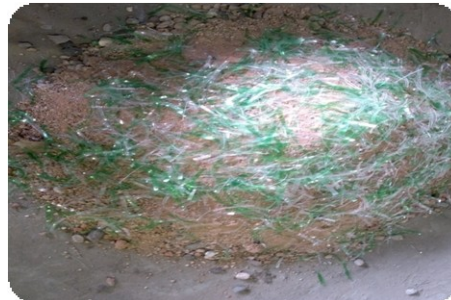
Figure 1. Waste plastic fibers mixed with other mixture components before mixing operation
