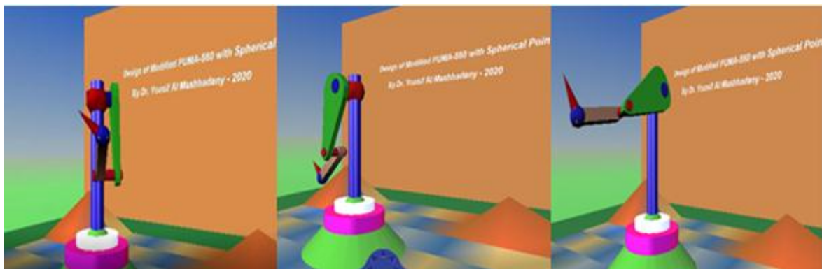
Figure 8. Postures of the modified PUMA 560 in different trajectories
