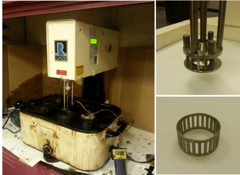
Figure 2. The Ross blending machine and its components
