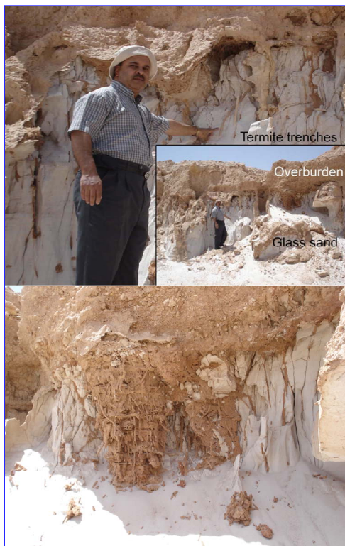
Figure 2. Network of termite trenches penetrating the overburden (brown color) and glass sand (white color).
