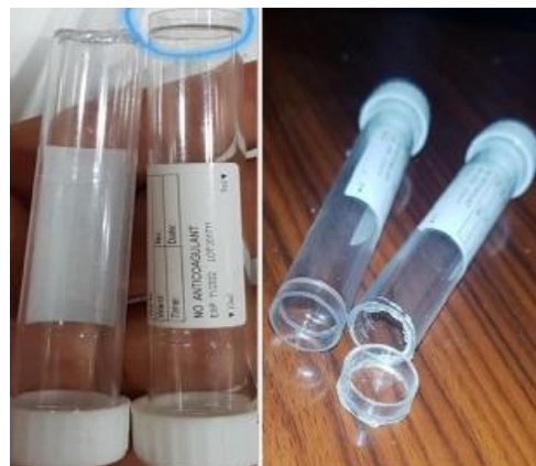
Fig. 1. Lower bottom of plane tube was cut and sterilized in order to use as a container for gas production
