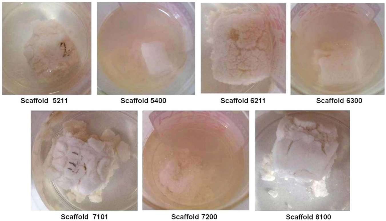
Fig. 12. Photographs show the degradation manner of each scaffold using PBS after 3 days.
