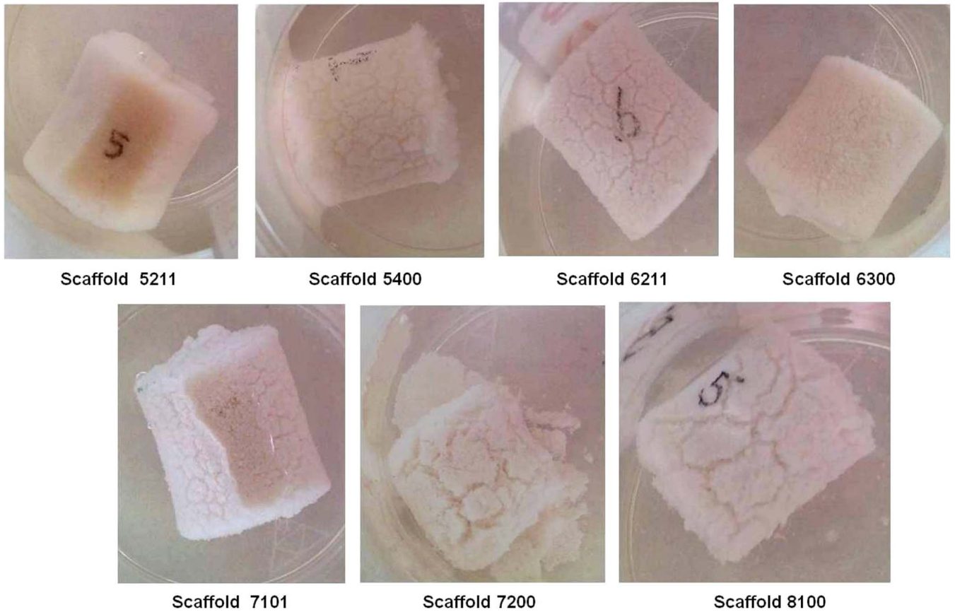
Fig. 11. Photographs show the degradation manner of each scaffold using PBS after 24 h.
