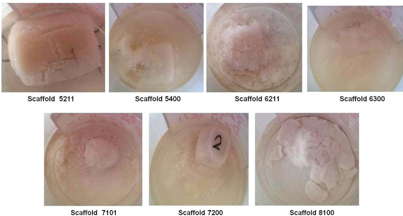
Fig. 10. Photographs show the degradation manner of each scaffold using Lysozyme after 7 days.
