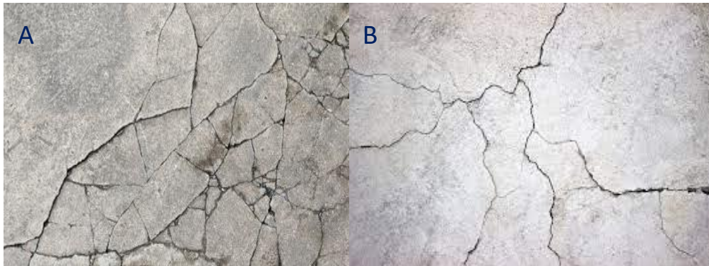
Figure (1): Small and micro-cracks of concrete under microscope; A: Before healing, B: after the addition of bacterial spores for healing activity.
