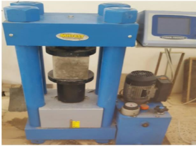
Figure 2: Cube test inside Compressive Strength Machine
