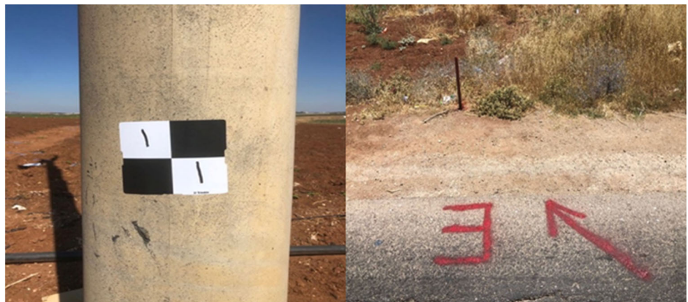
Fig. 3 Left: sample of tie points. Right: sample of ground control points
