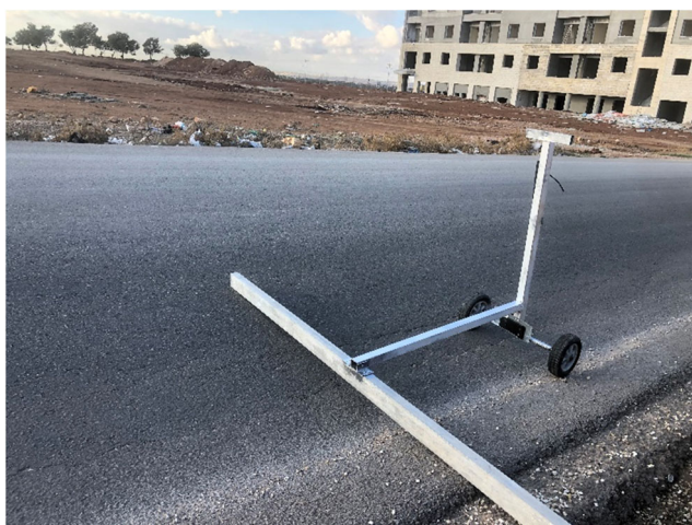
Fig. 5 Image pixel measurements tool for rutting measurements
