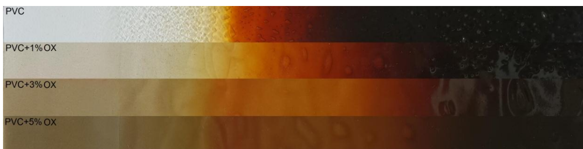
Figure 8.2. Static heat stability test at 190°C for plasticized poly(vinyl chloride) containing Oxydron (OX symbol)
