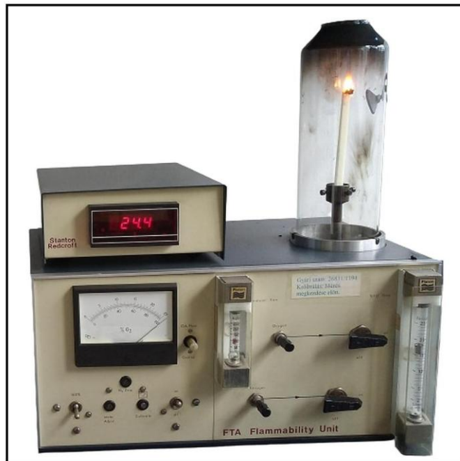
Figure 7.7. Stanton Redcroft FTA flammability unit
