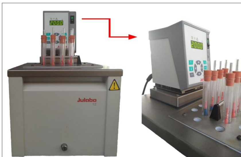
Figure 7.8. Julabo MC-12 circulator oil bath, and the test paper appears in orange and blue color
