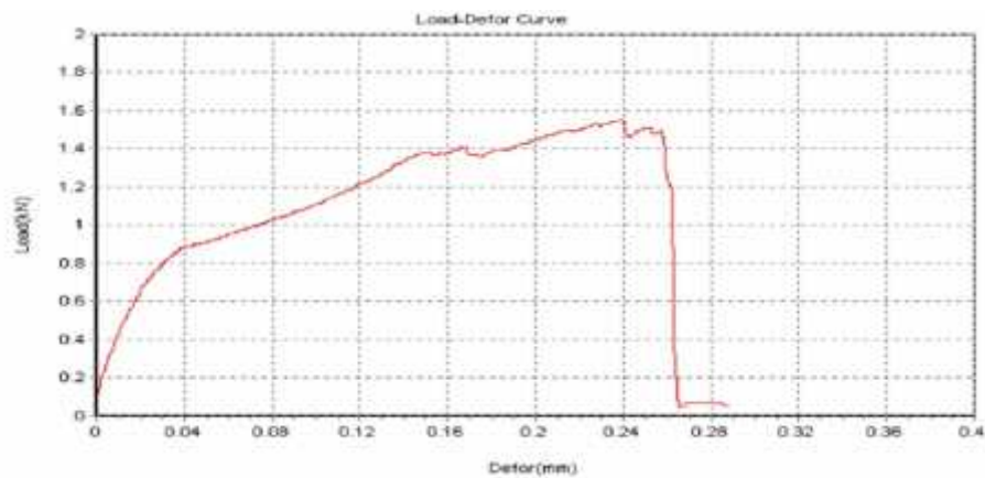
Figure 18 Tensile Strength curve of C alloy
