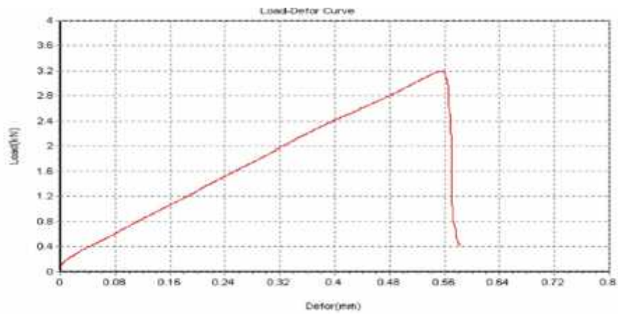
Figure 16 Tensile Strength curve of A alloy
