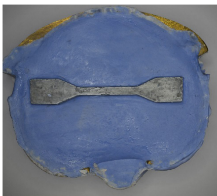
Fig1.Metal pattern located onto stone mould
