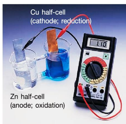
Figure 6-3 Measurement of a standard cell potential. The zinc-copper cell, operating at 298 K under standard-state conditions, produces a voltage of 1.10 V .
