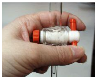
Figure 1.2. The proper handling of the stopcock of the burette. This allows for maximum control of the rate at which the titrant is added.
