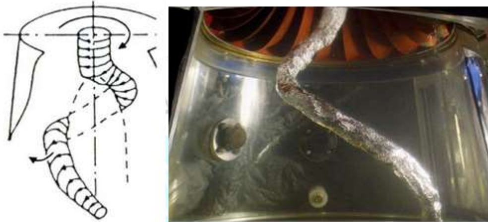
Figure 3: Dead water core (left), and draft tube vortex with a vapor core [1].
