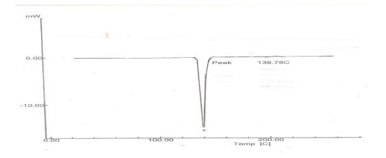
FIGURE 2. Typical Differential Scanning Calorimetric (DSC) profile for the Sn40-Bi60
