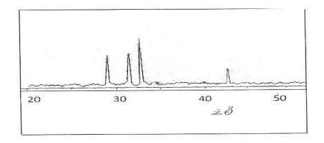
FIGURE 1. X-ray Diffraction Pattern of the Sn40-Bi60 alloy .
