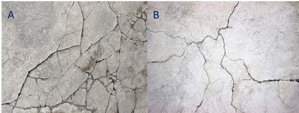
Figure (1): Small and micro-cracks of concrete under microscope; A: Before healing, B: after the addition of bacterial spores for healing activity.
