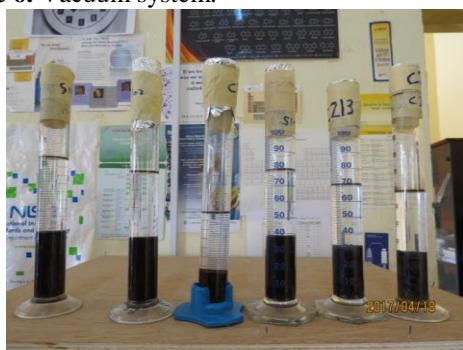
Figure 8. Close pipe orifice to prevent evaporation of oil
