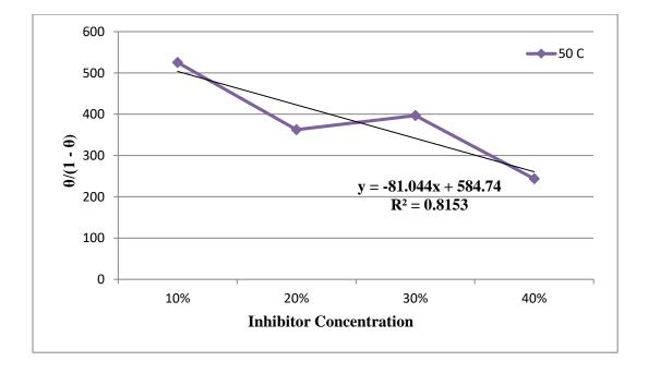
Fig. (3.6) : Langmuir Adsorption Isotherm of "Alcoholic Extract Moringa " Inhibitor on Mild Carbon Steel in 0.5 M  $H_2SO_4$  at 50 °C.
