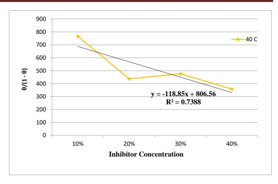
**Figure (3.5) :** Langmuir Adsorption Isotherm of "Alcoholic Extract Moringa "Inhibitor on Mild Carbon Steel in  $0.5 \text{ M H}_2\text{SO}_4$  at 40 °C.
