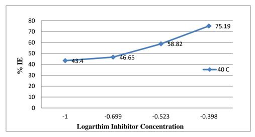
**Fig. (3.3)** The Variation Inhibition Percentage With the Logarithm of the Concentration of "Alcoholic Extract Moringa "Sulphur Containing Inhibitor Compound, at 40°C.
