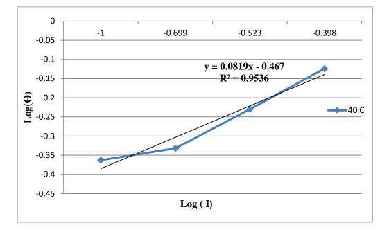
Fig. (3.9) : Freundlish Adsorption Isotherm of " Alcoholic Extract Moringa " Inhibitor on Mild Carbon Steel in 0.5 M  $H_2SO_4$  at 40 °C.
