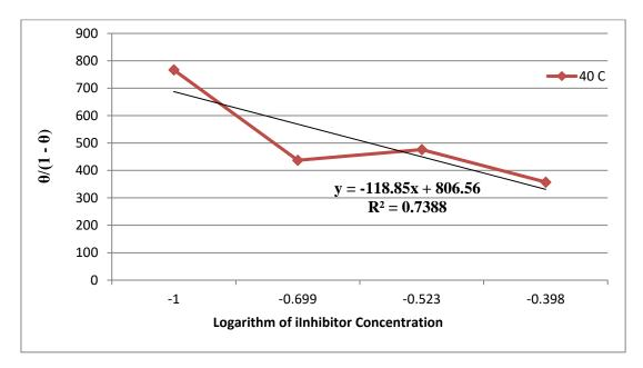
**Figure (3.7) :** Temkin Adsorption Isotherm of "Alcoholic Extract Moringa " Inhibitor on Mild Carbon Steel in 0.5 M H<sub>2</sub>SO<sub>4</sub> at 40 °C.
