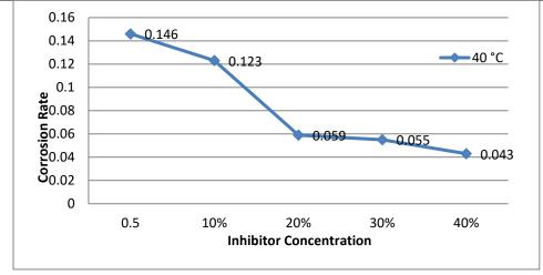
Fig. (3.1) The Relationship between Corrosion Rate and Inhibitor Concentration at 40C
