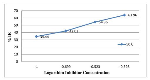
Fig. (3.4) The Variation Inhibition Percentage With the Logarithm of the Concentration of " Alcoholic Extract Moringa " Sulphur Containing Inhibitor Compound, 50°C
