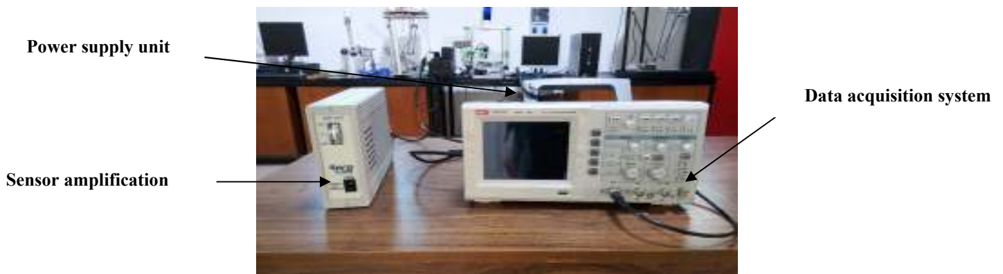
Fig. 2. Arrangement of equipment for an impact test.
