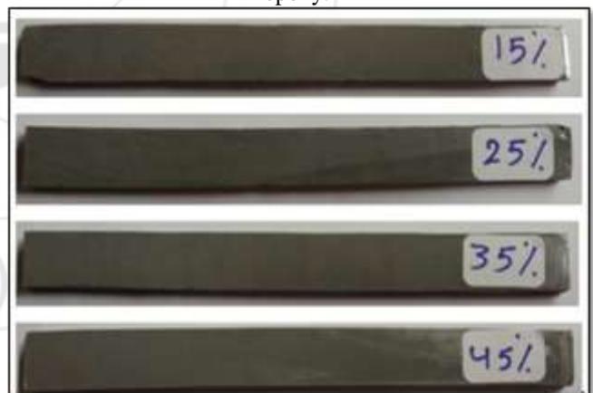
Figure (5): Photograph of Flexure Test Specimens for Epoxy/ Aluminum composites before testing
