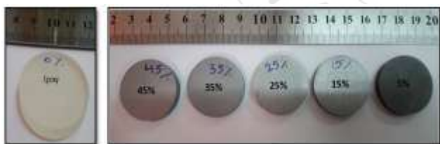
Figure 2: Photograph of Shore D Hardness Test Specimens for pure Epoxy and Epoxy/ Aluminum composites
