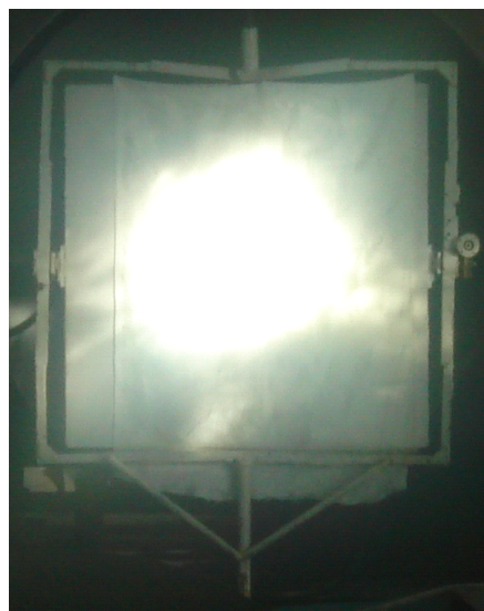
Figure. 8 Diffusely reflecting screen of the BSF, covered with a white heat-resistant cover.
